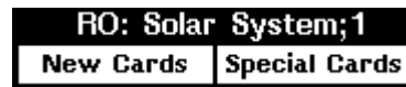
Figure 12-4. A notefile opened read-only with its Banner showing the read-only prefix "RO:"
